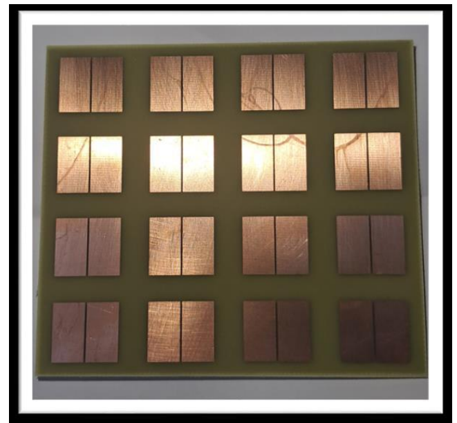
Figure 11. Fabricated 4 \times 4 RIS PCB array, showing the sixteen copper patch elements on FR4 substrate, each with a 0.5 mm central split-gap region prepared for varactor integration.
