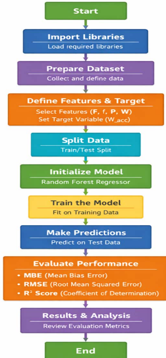
Figure 2: Characteristic Python algorithm for Random Forest Regressor for cement waste (WoGM) adoption
