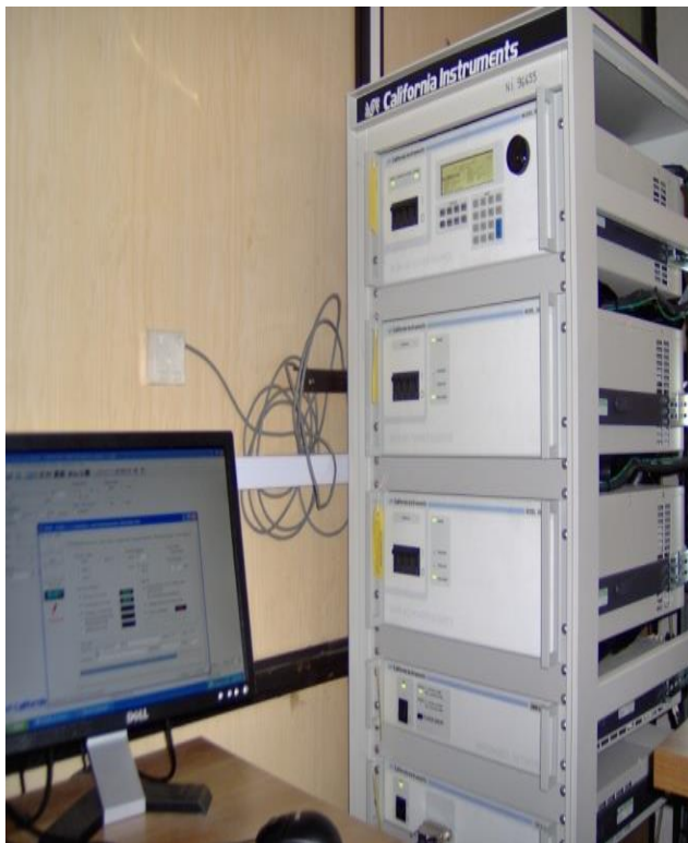
Fig. 7. Integrated test platform for modular multi-level DC-AC converters (MMCs)
