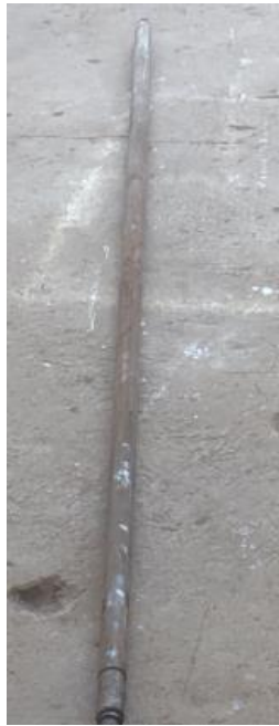
Figure 1.5 Sinker Bar 10 feet
