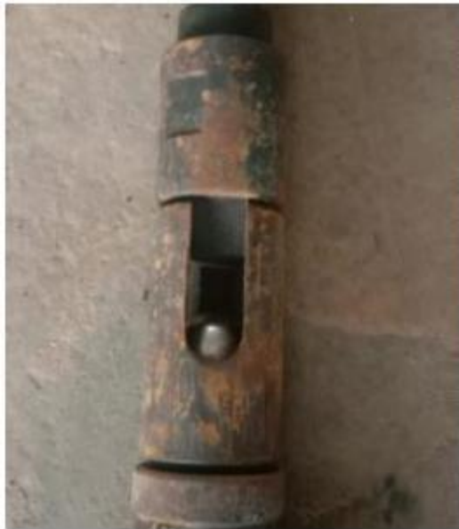
Figure 1.2 Cage Top TH Pump
