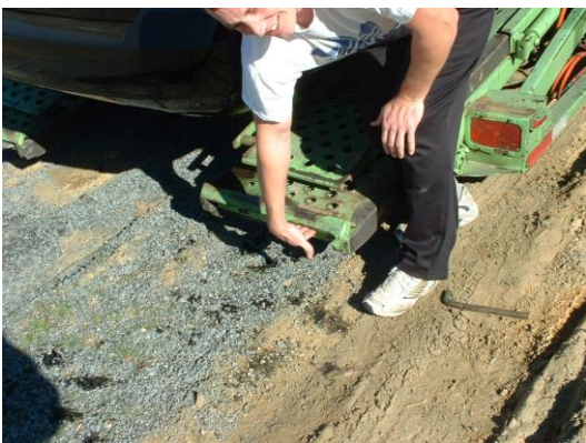
Figure 5 Fingers being smashed while retracting ramp.
