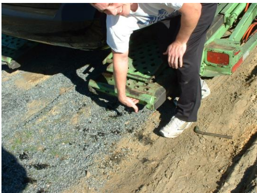
Figure 4 Fingers being smashed between ramp and ground
