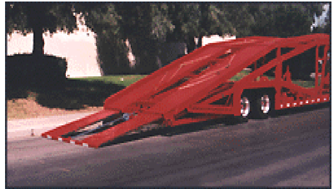
Figure 6 Hydraulic Loading Ramps on a Commercial Car Carrier
