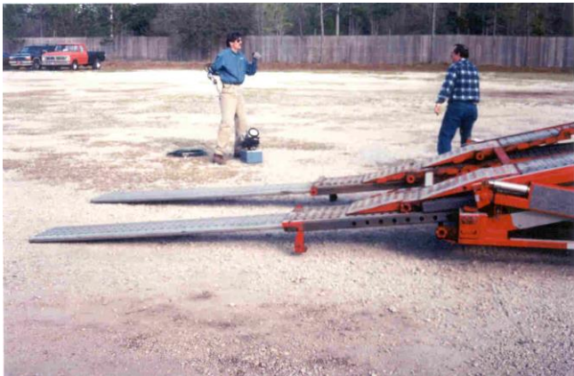
Figure 2: Side view of trailer with loading ramps fully extended
