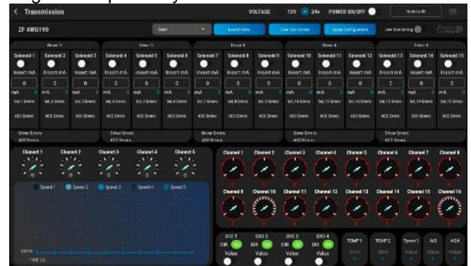
Fig. 29. HMI screen for transmission systems diagnosis and debug
