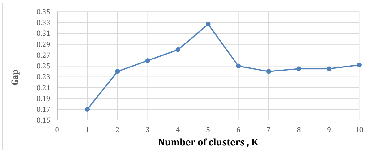
Figure 1 The graph for the gap analysis for determination of the number of cluster head, K required in the ELA-WF algorithm
