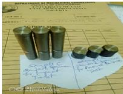
Impact strength and hardness test specimens for C 2
