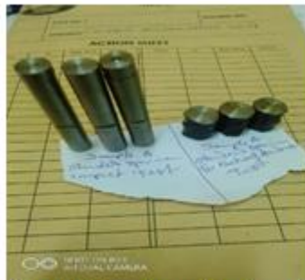
Impact strength and hardness test specimens for A 1
