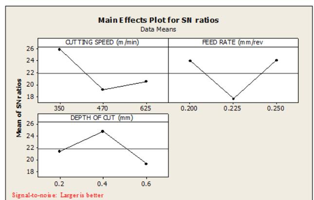
Fig. 5: Main effects plots for signal-to-noise (S/N) ratio
