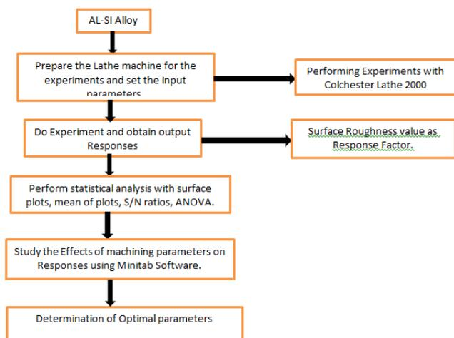
**Fig. 2** Flow chart showing optimization methodology for the dry cutting.
