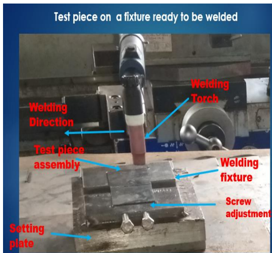
Plate 4: Specimen clamping on setting table
