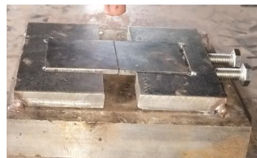
Plate 3: Workpiece clamping ready for TIG welding
