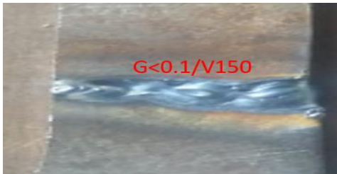
Plate 5: Welded sample for current of 100Amps, welding gap of 0.1mm and welding speed of 210mm/sec and 150mm/sec respectively.
