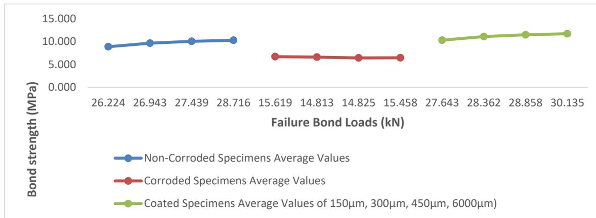
Figure 1a: Average Failure Bond loads versus Bond Strengths
