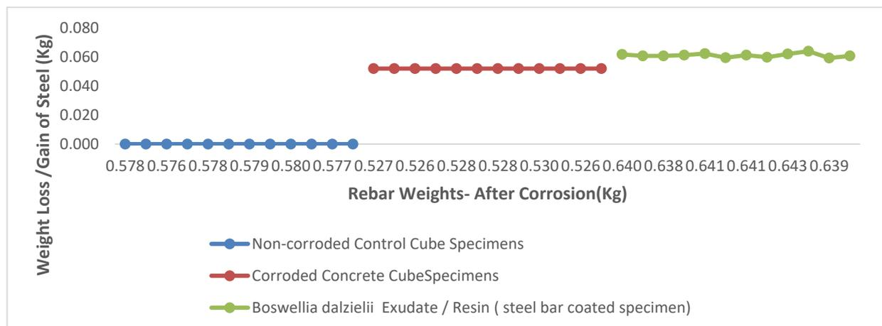
Figure 6: Rebar Weights- after Corrosion versus Weight Loss /Gain of Steel
