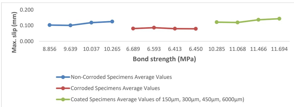
**Figure 2a: Average Bond Strengths versus Maximum Slip**
