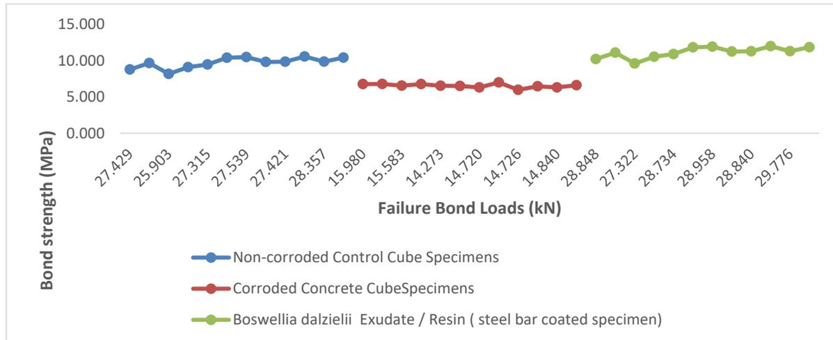
Figure 1: Failure Bond loads versus Bond Strengths
