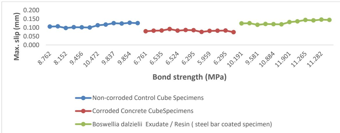
**Figure 2: Bond Strengths versus Maximum Slip**
