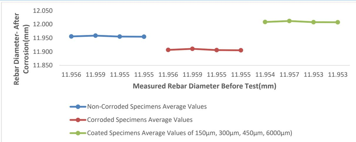
Figure 3a: Average Measured (Rebar Diameter before Test vs Rebar Diameter- after Corrosion)
