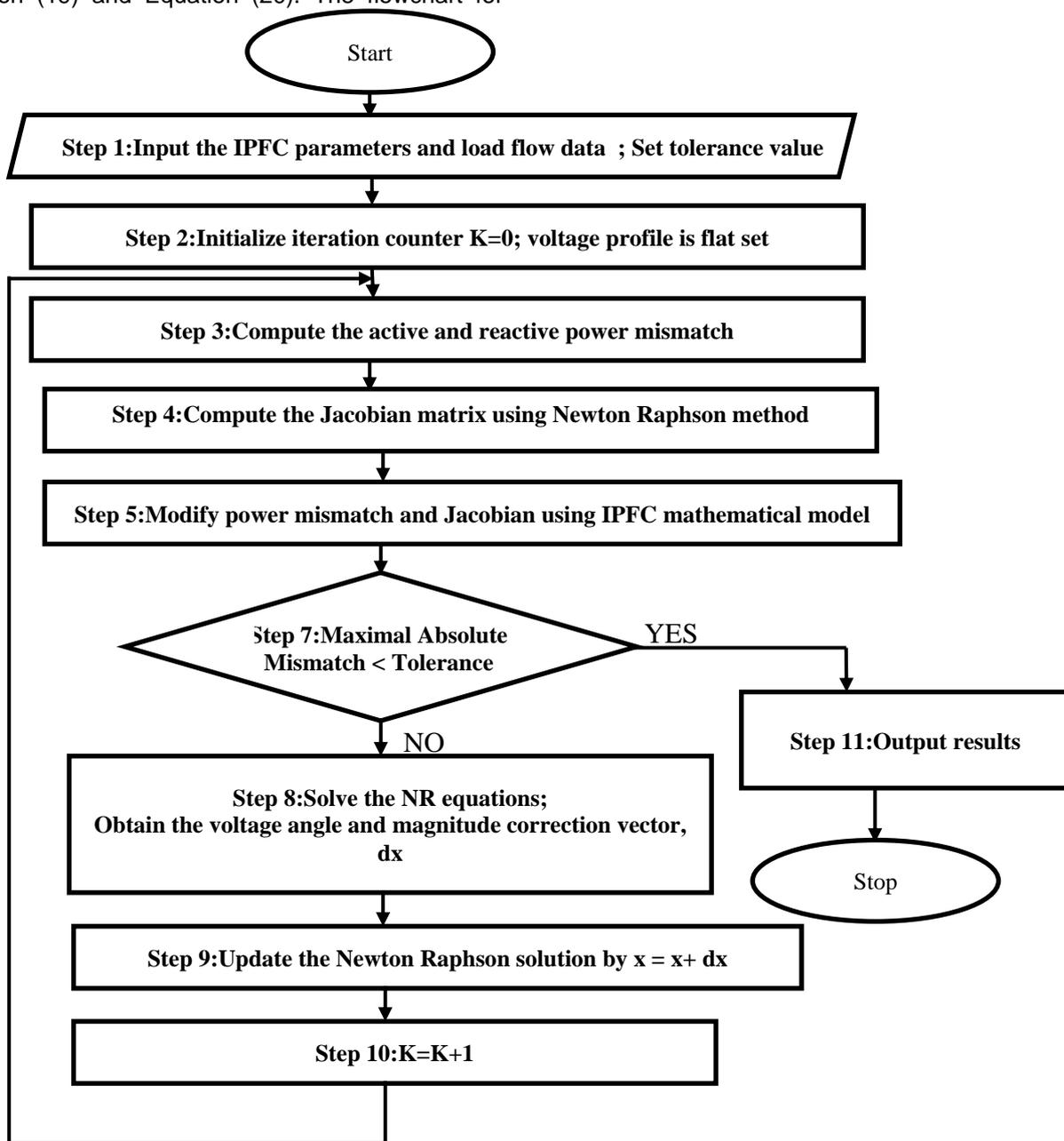
Figure 3 The flowchart for Newton-Raphson method with IPFC model
