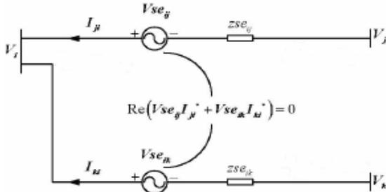
Figure 1 Equivalent circuit of two converter IPFC [34,35]
