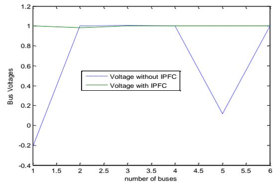
Figure 4, Voltage profile of buses with and without IPFC device
