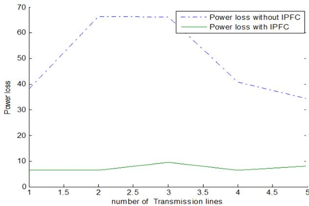
Figure 5: Plot of Power loss with and Without IPFC device.
