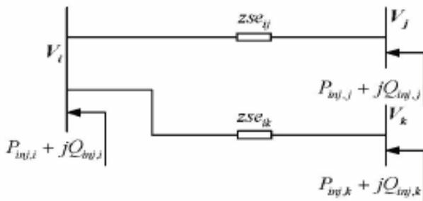
Figure 2: Power injection model of two converter IPFC
