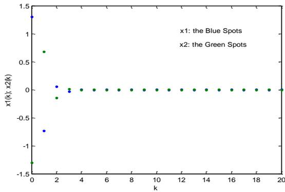
**Figure 1:** Typical state trajectories of system (5)-(6) with  $x(0) = [1.3 \ -1.3]^T$ .
