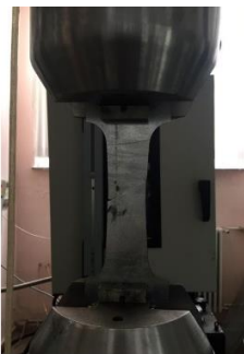
Fig. 5. Tensile test setup and testing procedures
