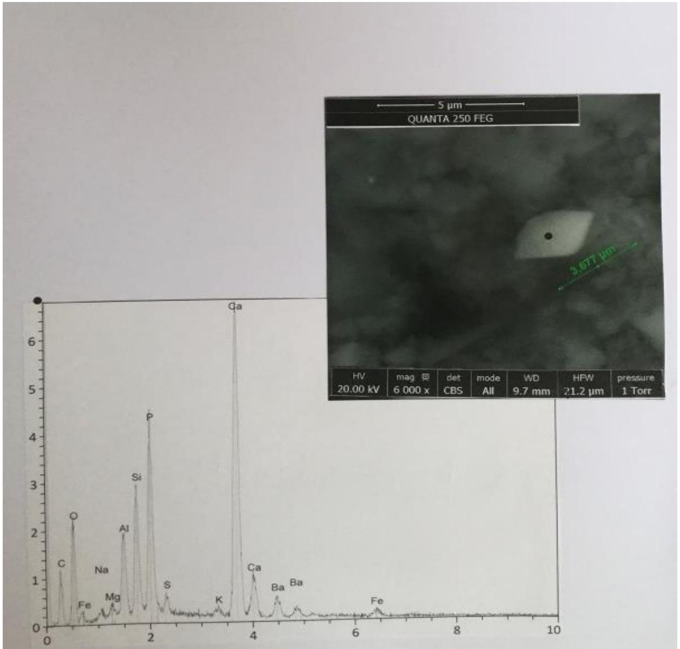
**Fig. 12** : A second example of barytine particle (1) – with another one (2), of more little size. *Above* : SEM photograph (in CBS, 6000x) of the particles 1 and 2. *Below* : spectrum at the black point. C : carbon ; O : oxygen ; Fe (two peaks) : iron ; Na : sodium ; Mg : magnesium ; Al : aluminium ; Si : silicium ; P : phosphorous ; S : sulphur ; K : potassium ; Ca (two peaks) : calcium ; Ba (two peaks) : barium.
