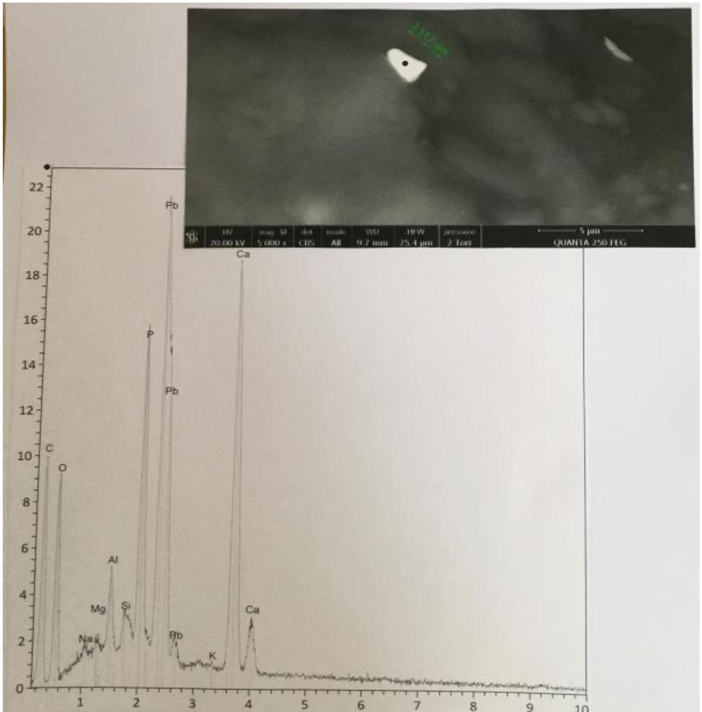
**Fig. 5 :** Above : SEM photograph (in CBS, 5000x) of particle number 4. Below : spectrum at the black point. C : carbon ; O : oxygen ; Na : sodium ; Mg : magnesium ; Al : aluminium ; Pb (three peaks) : lead ; K : potassium ; Ca (two peaks) : calcium ; Fe (traces) : iron .
