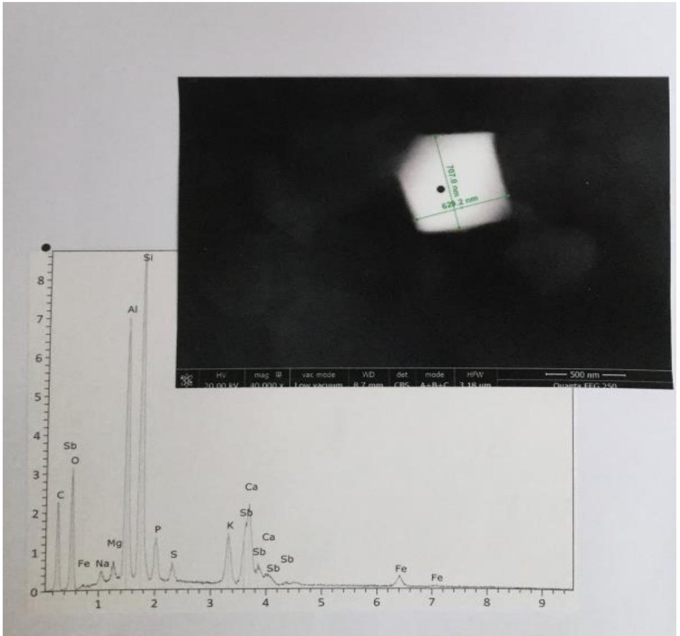
**Fig. 10 :** Above : SEM photograph (in CBS, 5000x) of the barium particle. Below : spectrum at the black point. C : carbon ; O : oxygen ; Fe (three peaks) : iron ; Na : sodium ; Mg : magnesium ; Al : aluminium ; Si : silicium ; P : phosphorous ; S : sulphur ; K : potassium ; Ca (two peaks) : calcium ; Ba (two peaks) : barium ; Ce (two peaks) : cerium.
