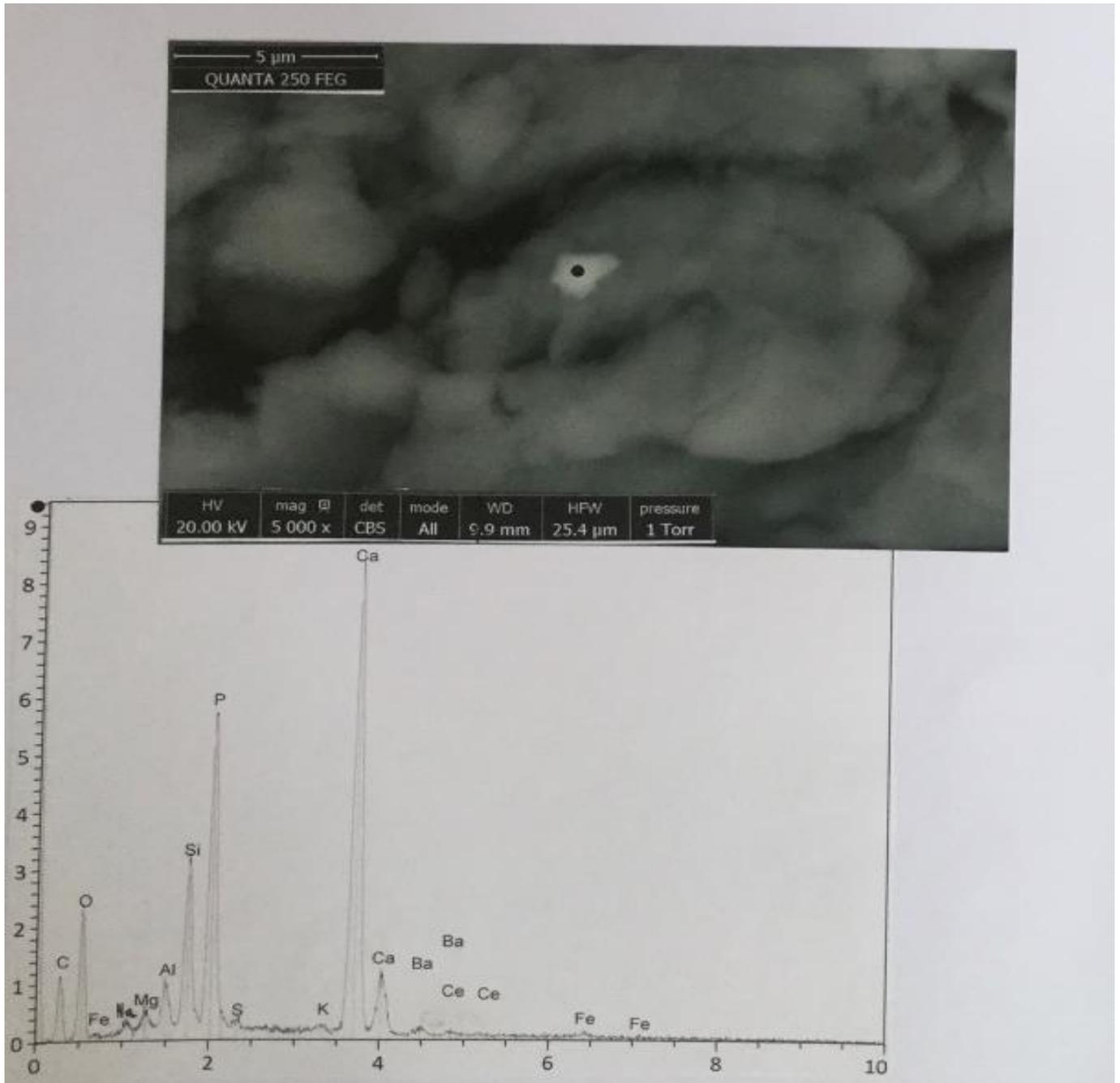
**Fig. 11** : A first example of a barytine particle, located on the lingual face of the tooth. *Above* : SEM photograph (in CBS, 6000x) of the particle. *Below* : spectrum at the black point. C : carbon ; O : oxygen ; Fe (two peaks) : iron ; Na : sodium ; Mg : magnesium ; Al : aluminium ; Si : silicium ; P : phosphorous ; S : sulphur ; K : potassium ; Ca (two peaks) : calcium ; Ba (three peaks) : barium.
