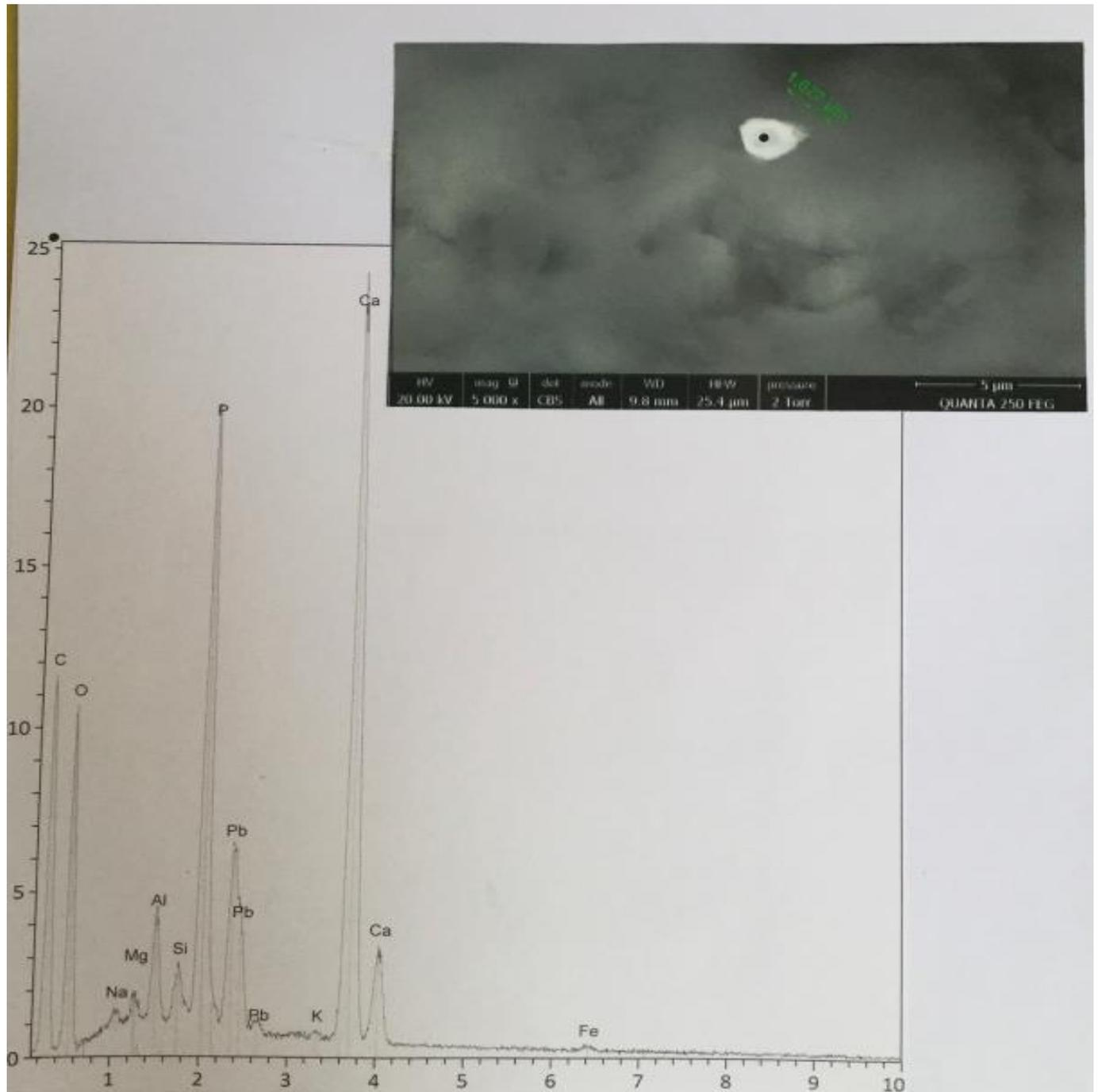
**Fig. 6 :** Above : SEM photograph (in CBS, 5000x) of particle number 7 (dimension is in nm). Below : spectrum at the black point. C : carbon ; O : oxygen ; Cu (two peaks) : copper ; Na : sodium ; Mg : magnesium ; Al : aluminium ; Si : silicium ; P : phosphorous ; Pb (three peaks) : lead ; K : potassium ; Ca (two peaks) : calcium ; Fe : iron.
