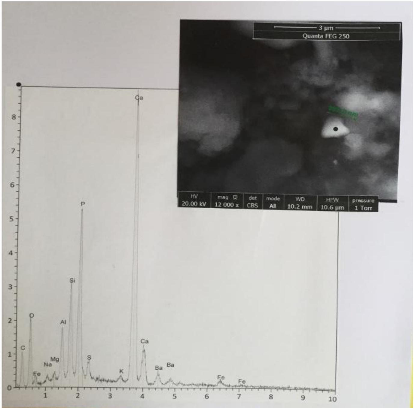
**Fig. 14** : A group of barytine particles of a powder . *Above* : SEM photograph (in CBS, 6 000x) of the group. *Below* : spectrum at the black point. C : carbon ; O : oxygen ; Fe (two peaks) : iron ; Na : sodium ; Mg : magnesium ; Al : aluminium ; Si : silicium ; P : phosphorous ; S : sulphur ; K : potassium ; Ca (two peaks) : calcium ; Ba (four peaks) : barium. The main ray of cerium is indicated.
