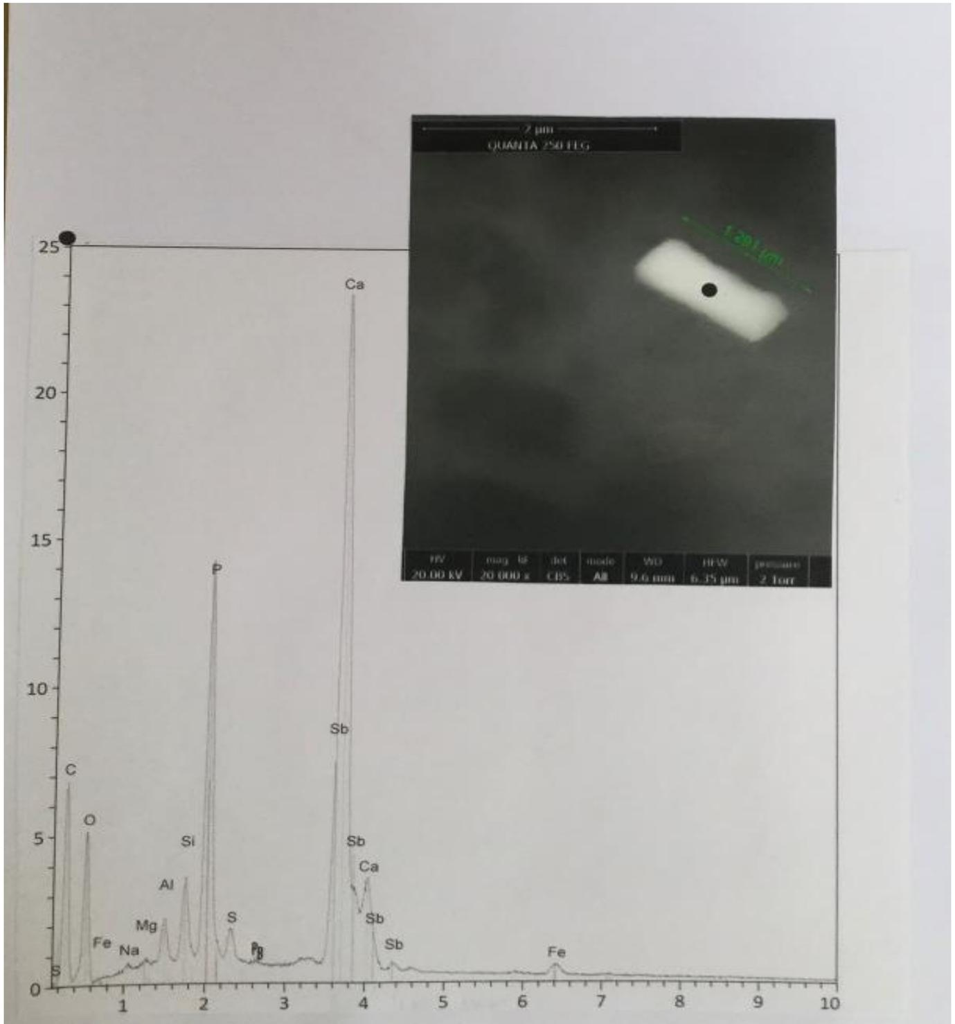
**Fig. 9** : A crystal of antimony sulphide, located on the lingual face of the tooth. *Above* : SEM photograph (in CBS, 40 000x) of the crystal. *Below* : spectrum at the black point. C : carbon ; O : oxygen ; Fe (three peaks) : iron ; Na : sodium ; Mg : magnesium ; Al : aluminium ; Si : silicium ; P : phosphorous ; S : sulphur ; K : potassium ; Ca (two peaks) : calcium.
