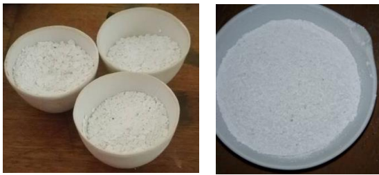
Fig.4.Calcined eggshells until turned white at various temperatures
