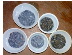
Fig.5.Calcined eggshells at various temperatures for 1 hour.
