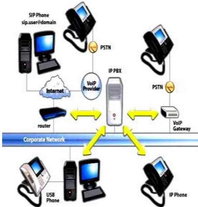
Figure 1: Architecture of Voice over Internet Protocol. (Source: Jalendry & Verma, 2015).
