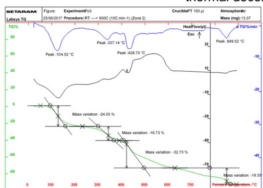
Fig 1. Thermal gravimetric analysis (TGA) of bagasse
