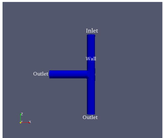
Figure 5: Schematic of Boundary Condition of the pipe for Case 2
