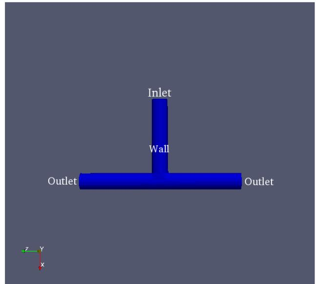
Figure 4: Schematic of Boundary Condition of the Pipe for Case 1
