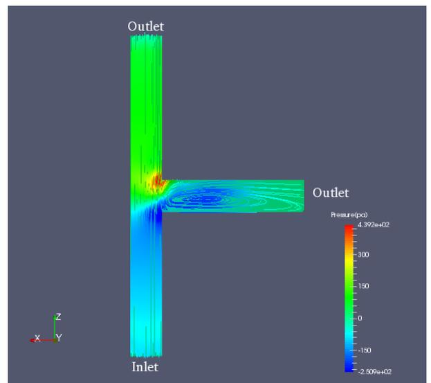
Fig 8: Velocity contour in m/s for case 2
