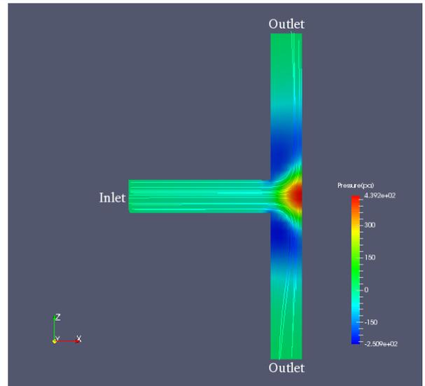
Fig 7: pressure contour for case 1
