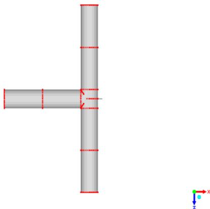
Figure 3: FEA Model of the Te-junction Pipe showing Nodes and element surface
