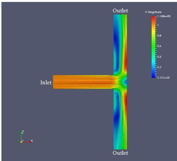
Fig 6: Velocity Contour in m/s for case 1
