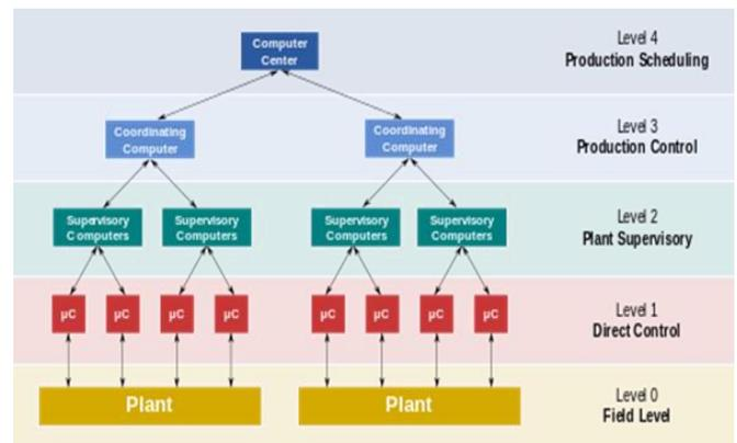
Fig. 4. Functional levels of a manufacturing control operation
