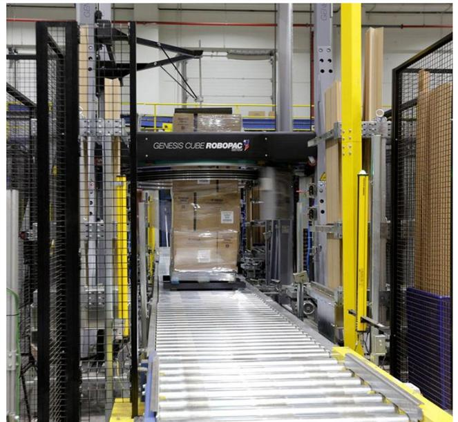
Fig. 6. Pallet wrapping process
