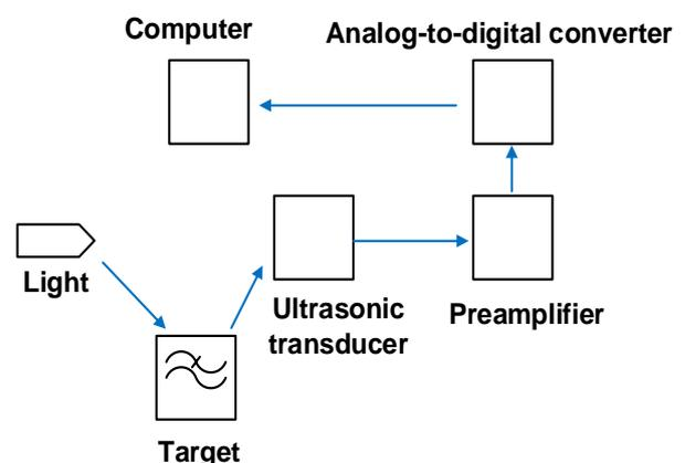
Fig. 1. Basic configuration of photoacoustic systems.
