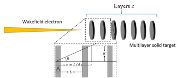
Fig.8 Schematic diagram of multilayer targets structure
