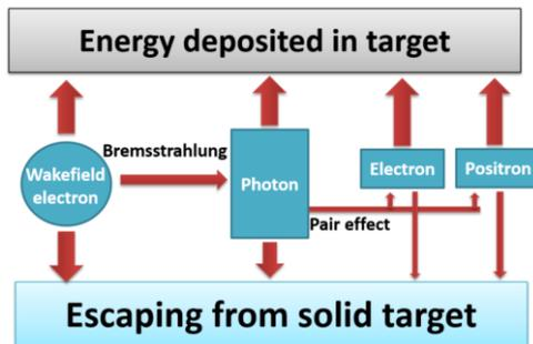
Fig.1 Transport process of wakefield electrons in target
