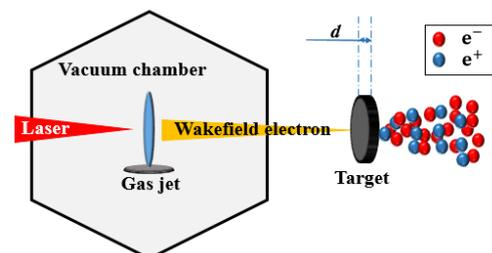
Fig.3 Positrons generation driven by laser under single Target
