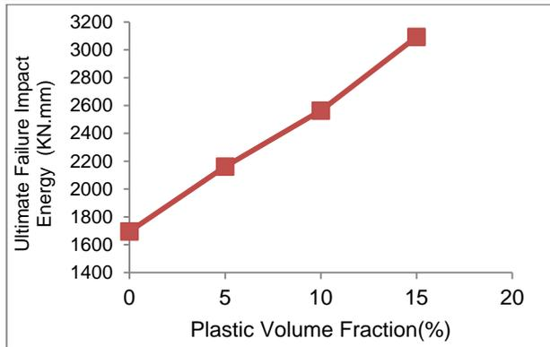
Fig. 8. Ultimate failure impact energy against volume fraction of plastic.
