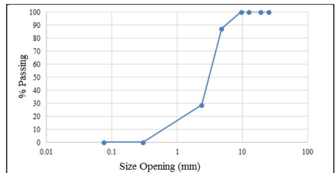
Fig. 2. Particle size distribution of plastic waste.
