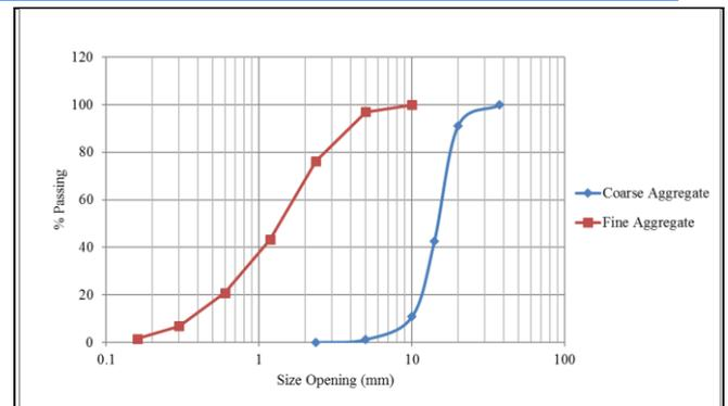
Fig. 1. Fine and coarse aggregates grading.
