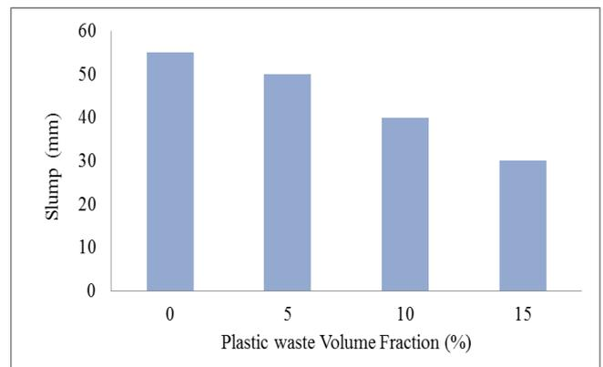
Fig. 5. Effect of sand replacement ratio on slump of plastic concrete.
