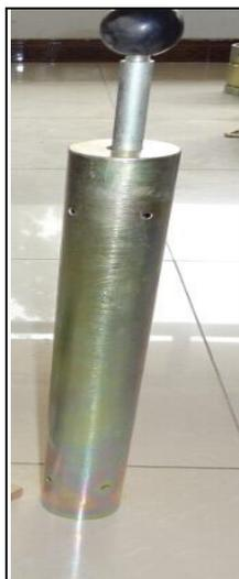
Fig. 4. Hammer of modified proctor.
