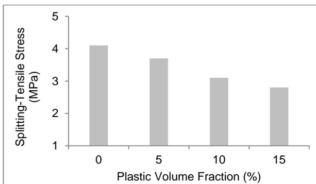
Fig. 6. Splitting tensile stress against volume fraction of plastic waste.
