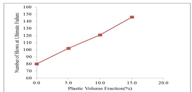
Fig. 7. Ultimate failure impact resistance against volume fraction of plastic.
