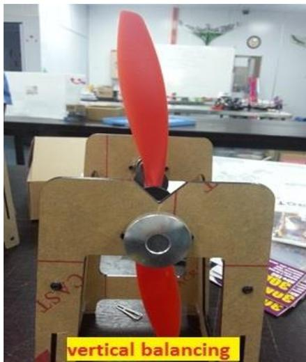
Fig. 2: Propeller balancing
