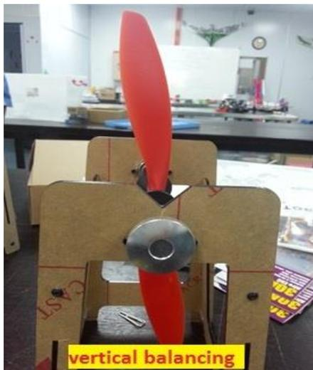
Fig. 2: Propeller balancing
