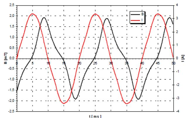
Fig.5. Time behaviors of B and IU for  $T=0.6 \text{ N.m}$ .
