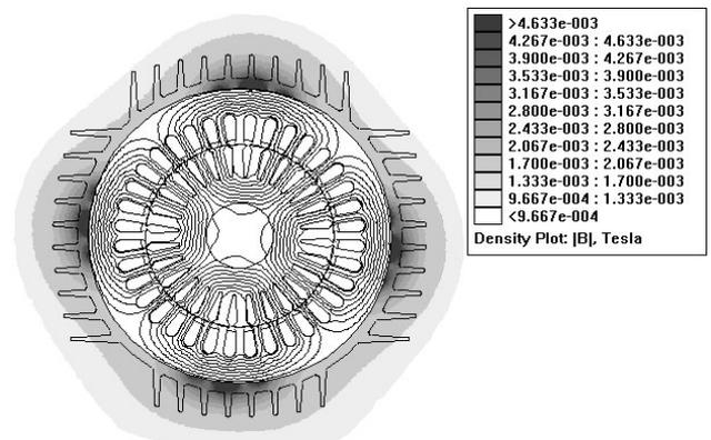
Fig.2. Static analysis of induction motor leakage field
