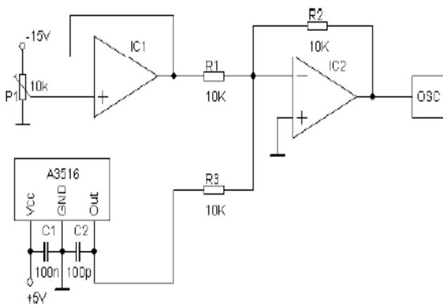
Fig .4.General View of circuit for time behaviors' of magnetic flux density measurement.
