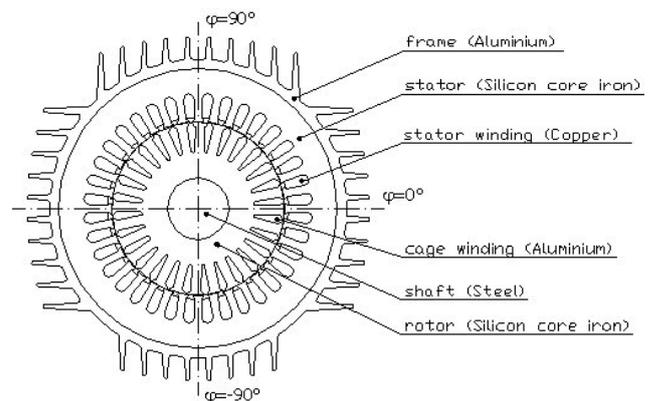
Fig.1. 2D induction motor mode
