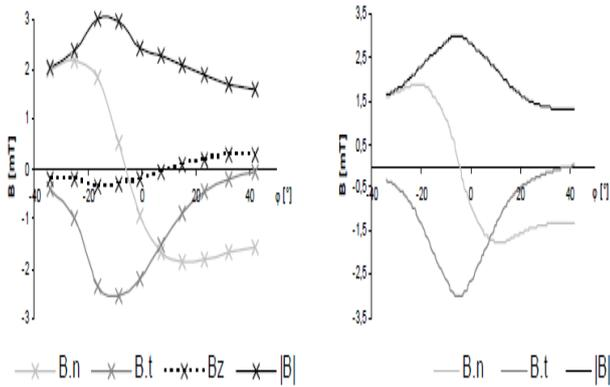
Fig.3. Magnetic flux density distribution above the Frame of motor.
