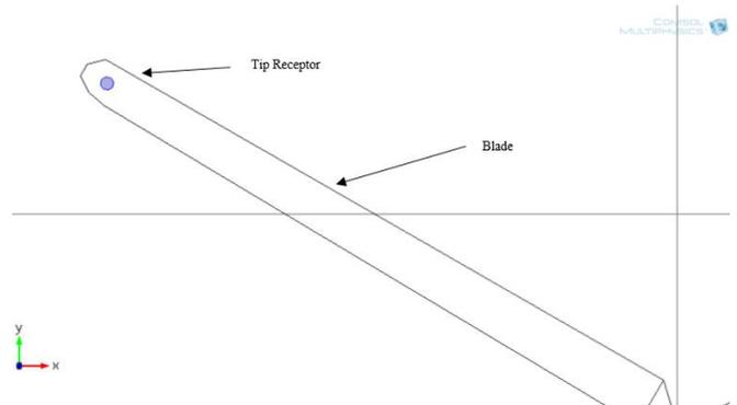
Figure 3. Wind Turbine Blade and the Tip Receptor
