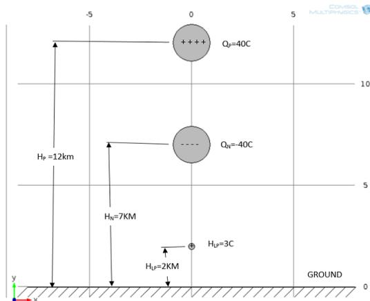
Figure 1. A vertical tri-pole made from two positive charges and a negative charge representing the idealized gross charge structure of a thundercloud. [15]
