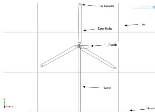
Figure 2. Wind Turbine Model
