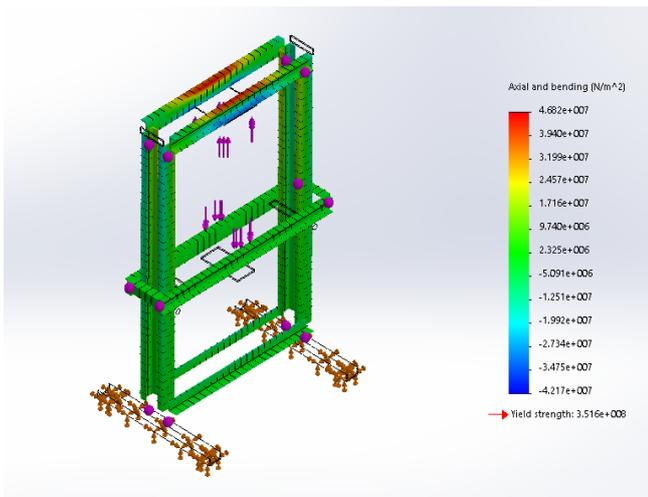
Fig. 6: Stress distribution of the designed hydraulic press frame when subjected to maximum loading condition
