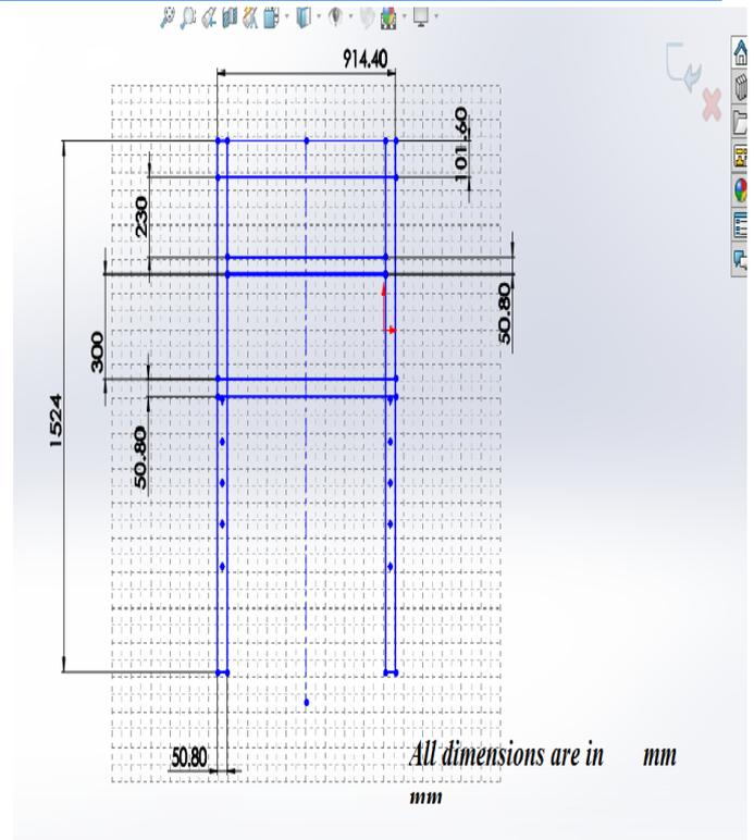
Fig. 4: A 2-d model of the designed frame showing general framework dimensions
