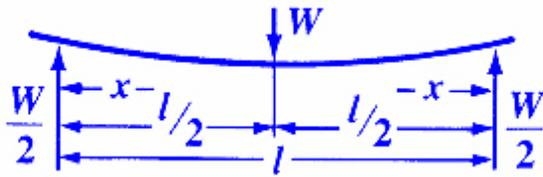
Fig. 2: Deflection for a beam supported at both ends with load at the centre
