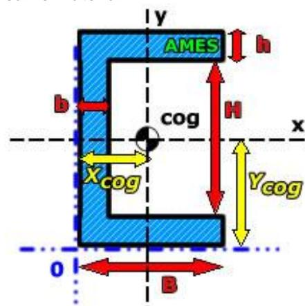
Fig. 1: sectional properties of c-channel beam
