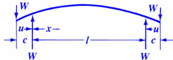
Fig. 3: Structural beam deflection for a beam with ends overhanging, support and two equal loads applied at symmetrical locations.
