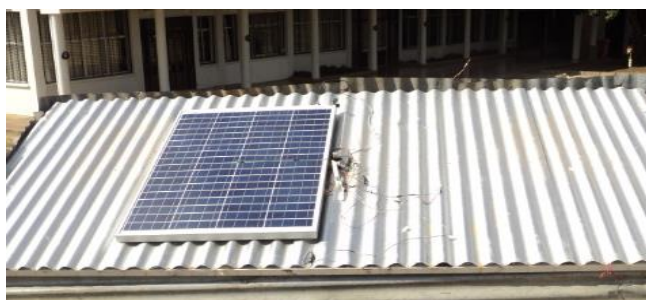
Fig. 3: Experimental setup: PV module attached to CMS and temperature sensors
