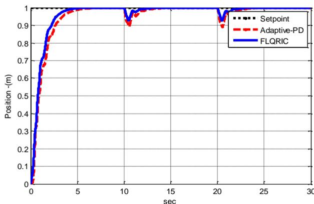
Fig. 9. Response of TWMR using an adaptive PD and FLQRIC for sine wave setpoint
