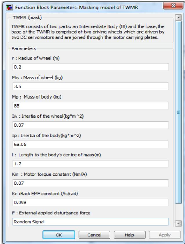
Fig. 1. Masking simulink model of the TWMR
