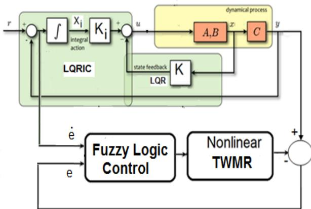
Fig. 5. Fuzzy state feedback with integral controller for TWMR
