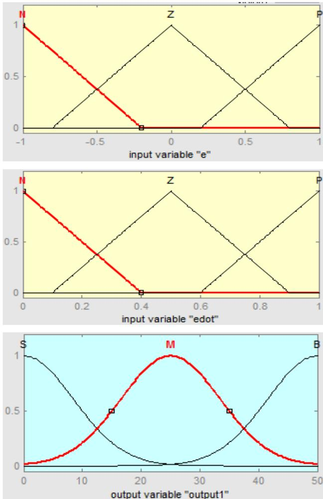
Fig. 6. Input and output membership functions for FLQRIC
