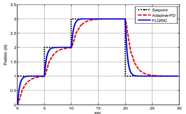
Fig. 8. Response of TWMR using an adaptive PD and FLQRIC for different level setpoint
