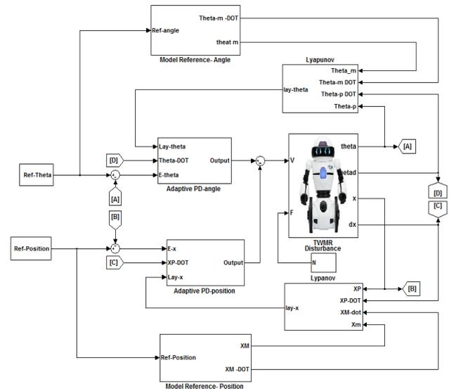
Fig. 4. Simulink model of adaptive controllers with TWMR
