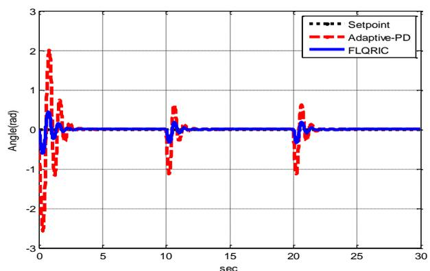
Fig. 10. Response of TWMR using an adaptive PD and FLQRIC with noise signal
