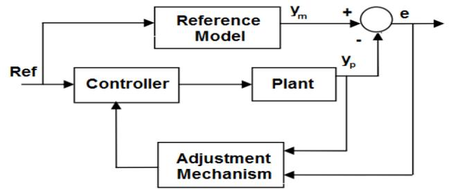
Fig. 2. Model reference adaptive controller
