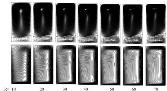
Figure 6: Streamlines of the secondary flow (top) and axial flow (bottom) in each row at different Rotation parameter where  $D_n = 1000, D_a = 0.1$ .
