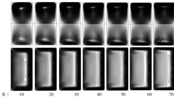
Figure 7: Streamlines of the secondary flow (top) and axial flow (bottom) in each row at different Rotation parameter where  $D_n = 1000, D_a = 1000$ .
