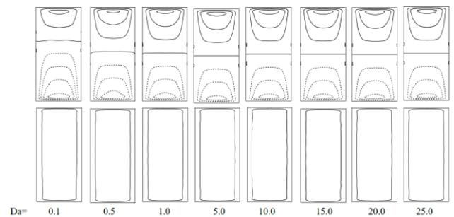
Figure 3: Streamlines of the secondary flow (top) and axial flow (bottom) in each row at different Darcy number where the Dean number and rotation parameter is treated as constant. ( $D_n = 100 \text{ and } R = 500$ ).
