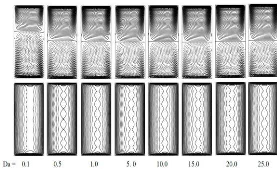
Figure 5: Streamlines of the secondary flow (top) and axial flow (bottom) in each row at different Darcy number where  $D_n = 1000, R = 500$ .
