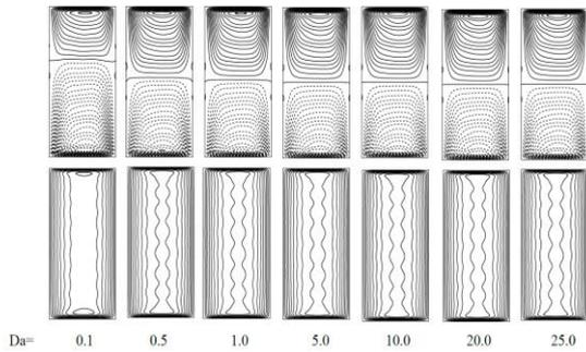
Figure 4: Streamlines of the secondary flow (top) and axial flow (bottom) in each row at different Darcy number where  $D_n = 500, R = 500$ .
