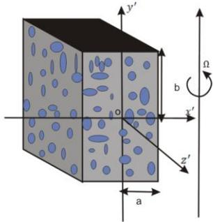
Figure 1: Geometrical configuration of the rectangular straight duct in the Darcian porous medium.
