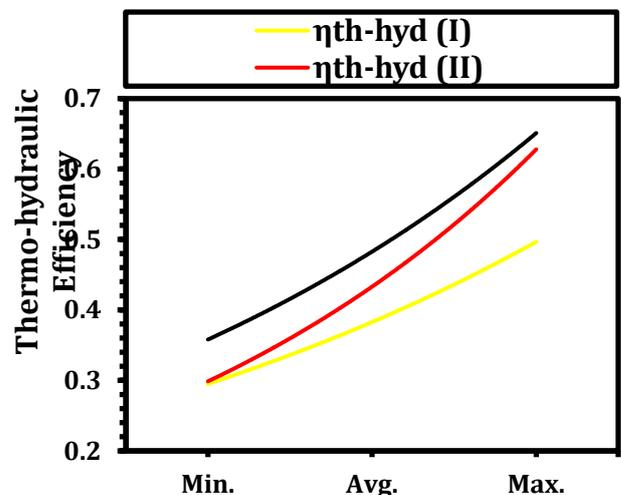
Fig. 7 Comparison in thermo-hydraulic efficiency of all models of SAC at 0.0139 kg/s
