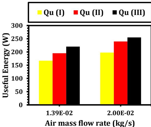
Fig. 9 Effect of air mass flowrate on average useful energy of air for all models
