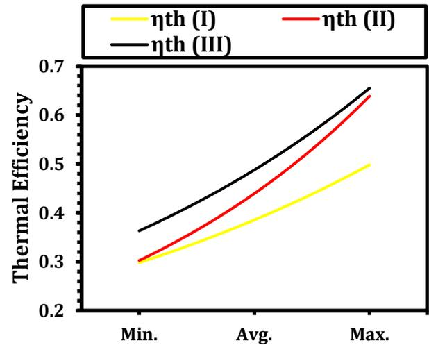
Fig. 6 Comparison in thermal efficiency of all models of SAC at 0.0139 kg/s
