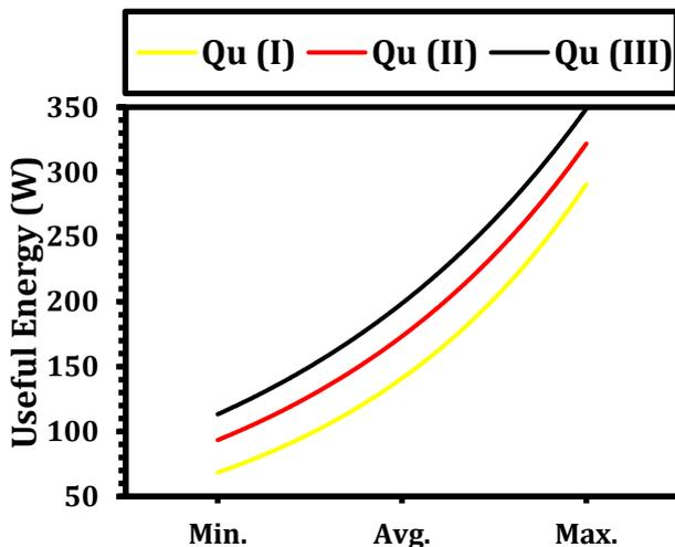
Fig. 5 Comparison in useful energy of air for all models at 0.0139 kg/s
