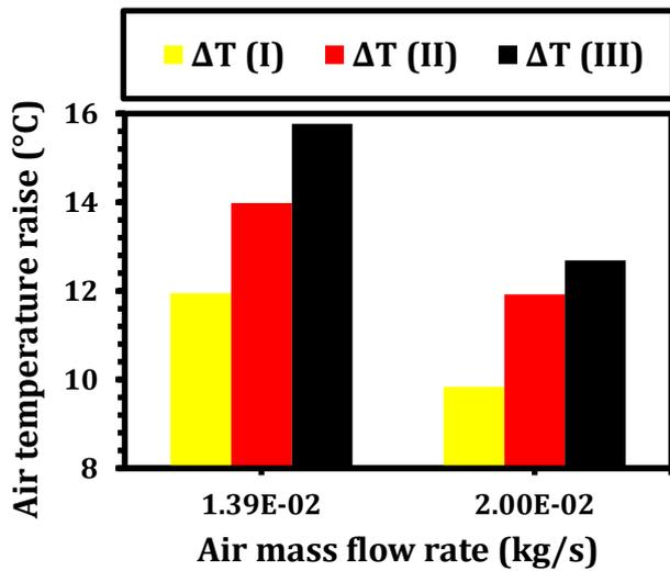
Fig. 8 Effect of air mass flowrate on average air temperature raise for all models
