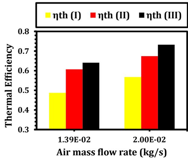
Fig. 10 Effect of air mass flowrate on average thermal efficiency of SAC for all models
