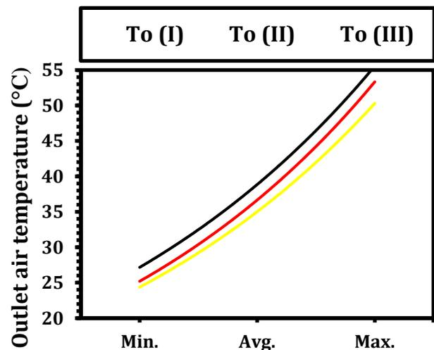
Fig. 3 Comparison in outlet air temperature for all models at 0.0139 kg/s
