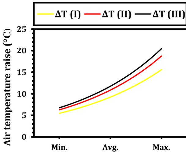
Fig. 4 Comparison in air temperature raise for all models at 0.02 kg/s
