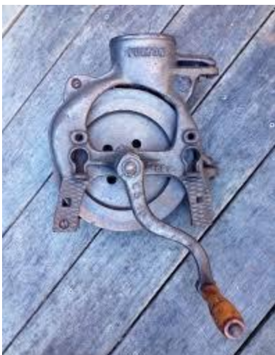
Figure 2.10: Antique Maize sheller
