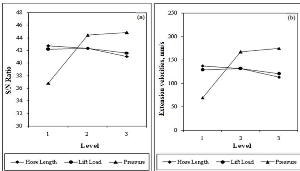
Fig. 2. Plots showing the mean effects of response for double acting cylinder, (a) S/N ratios, (b) Extension velocities
