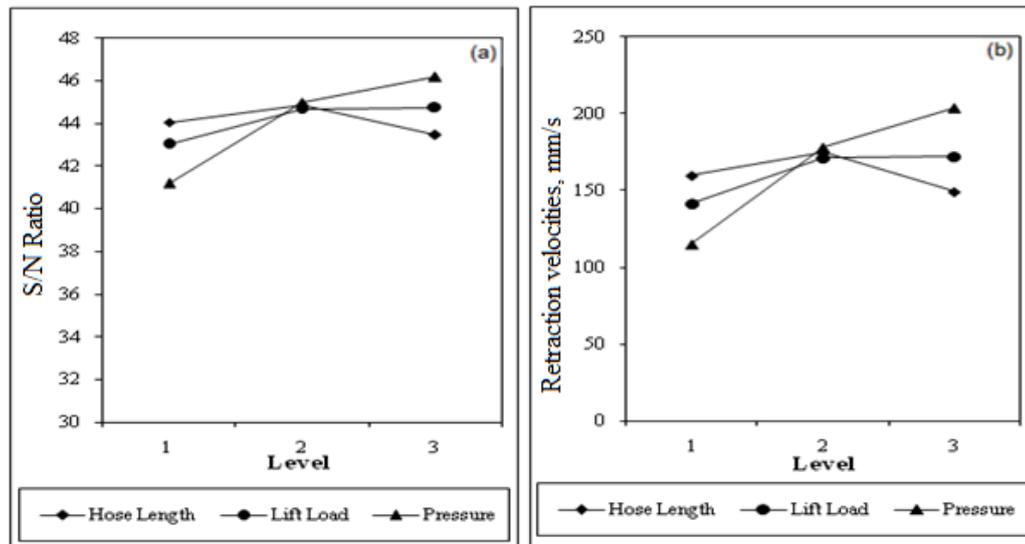
Fig. 3. Plots showing the mean effects of responses for double acting cylinder, (a) S/N ratios, (b) Retraction velocities
