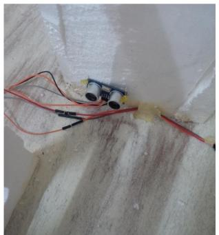
Fig.5: Ultrasonic Sensor
