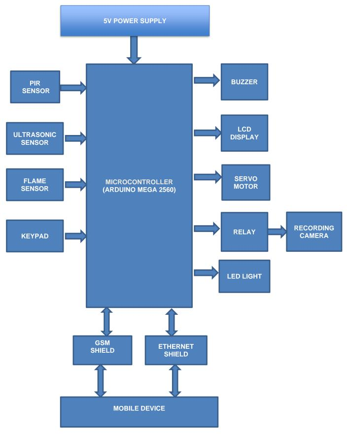
Fig.1: Architecture of the proposed system
