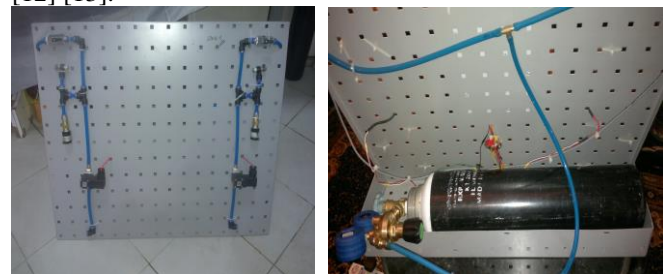
Fig.8 – (Front & Back) Experimental system Chassis with the O 2 cylinder for the Testing
