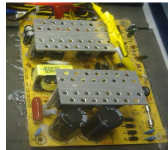
Fig.3– switching Mode Power supply
