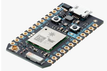
Fig.9 – Wi-Fi connected micro controller called “Photon Particle board”
