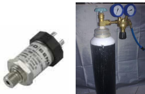
Fig.4 –a) BD digital pressure sensor; b) Oxygen Cylinder Tank with double stage regulator
