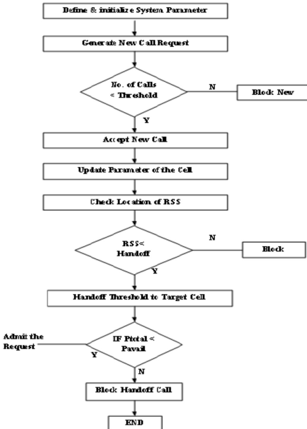
**Fig. 3. Flow Chart for CAC Handoff Prioritization Algorithm**
