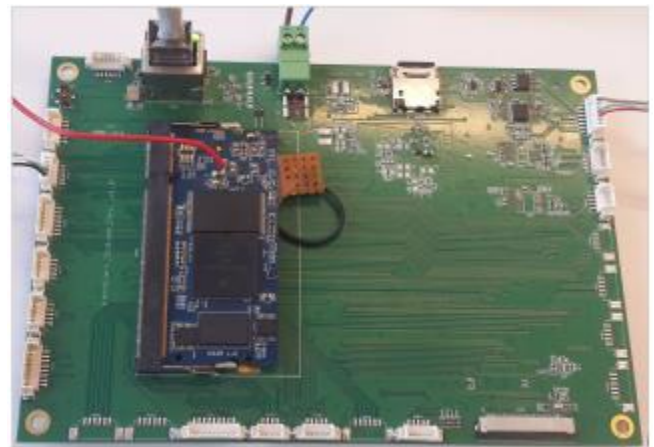
Fig. 8. Designed Sodimm module development set-up.
