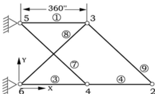
Fig. 2. The Optimized Ten-Bar Truss
