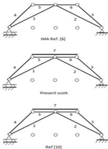
Fig. 6. The Optimized Ten-Node Truss ground structure
