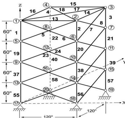
Fig. 4. The optimized 72-Bar Truss
