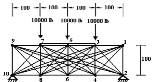
Fig. 5. Ten-Node truss ground structure
