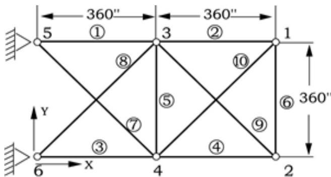
Fig. 1. The Ten Bar Truss
