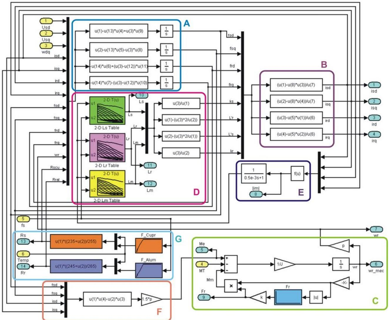
Fig. 4. Programming model of an asynchronous motor with cage rotor in the MATLAB/SIMULINK environment for high speed.
