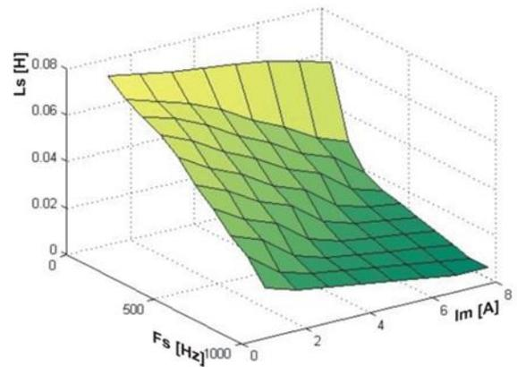
Fig. 1. Tabular function of the stator inductance.
