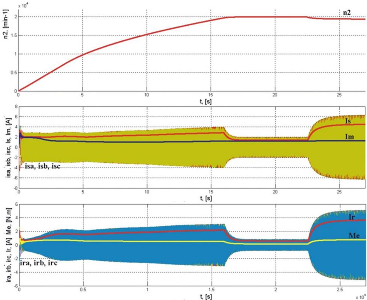
Fig. 5. Transitional processes in smooth start simulation and load of high-speed asynchronous motor ATF 80 E4 IM B3 with cage rotor and 4-pole at  $f_s=666,67\text{Hz}$ ,  $n_s=20000\text{rpm}$ .
