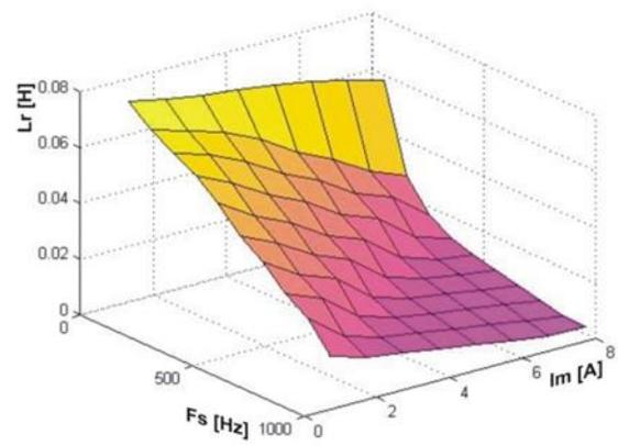
Fig. 2. Tabular function of the rotor inductance.
