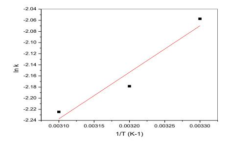
Fig.2 Temperature dependence of reaction rate
