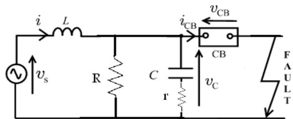
Fig 7. Circuit diagram with BR.
