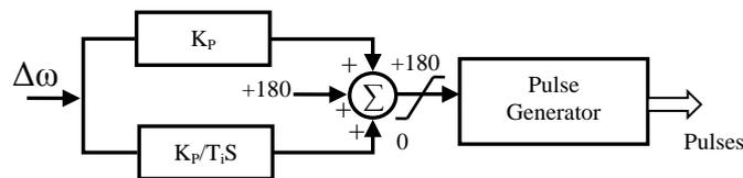
Figure 3. Block diagram of PI controller.
