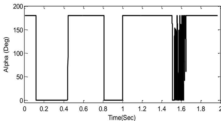
Figure 11. Firing angle for phase 'a'.
