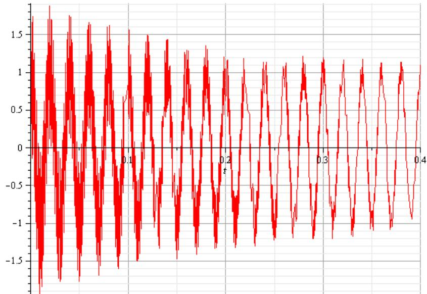
Fig 5. TRV voltage for a circuit without BR.
