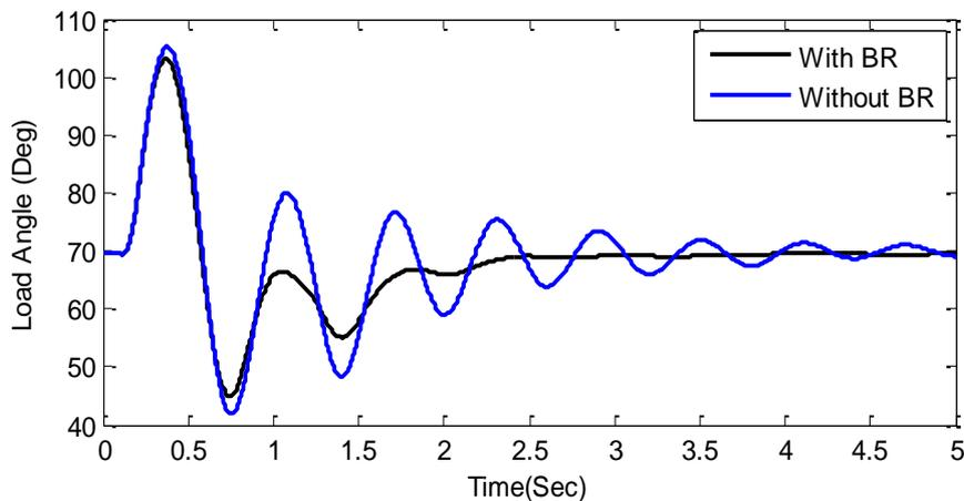
Figure 10. Load angle responses for 3LG fault.
