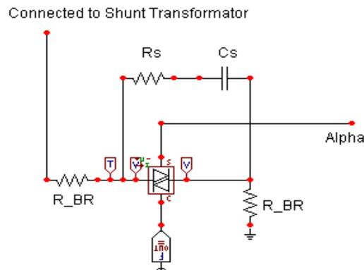
Figure 2. Phase 'a' related to BR, modeled in EMT/ATP.
