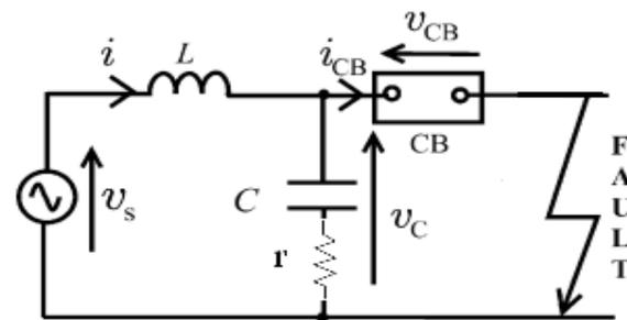
Fig 4. Simplified TRV circuit
