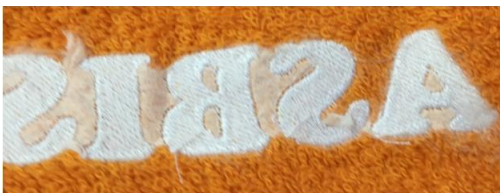
Fig. 8. Improper removal of the padding.
