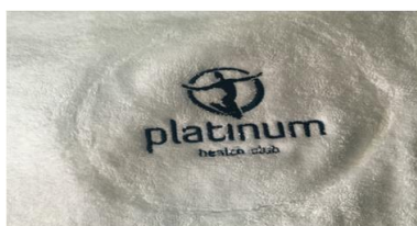
Fig. 9. Defect from the embroidery frame.
