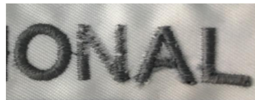
Fig. 3. Bobbin thread visible in the embroidery's surface.
