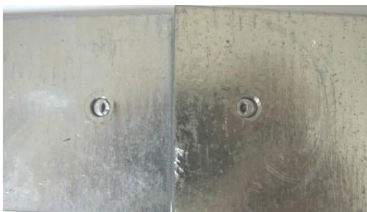
Fig. 11. Riveted joint after tensile test
