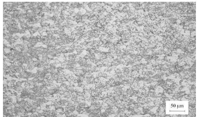
Fig. 2. Structure of S250GD steel sheet
