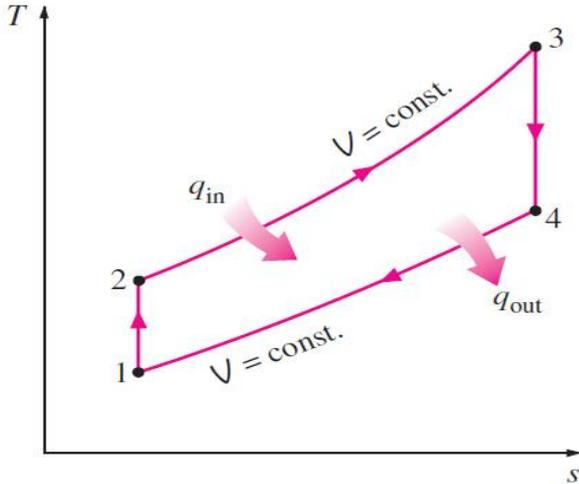
Fig. 1 The T-s diagram of air-standard Otto cycle [1]
