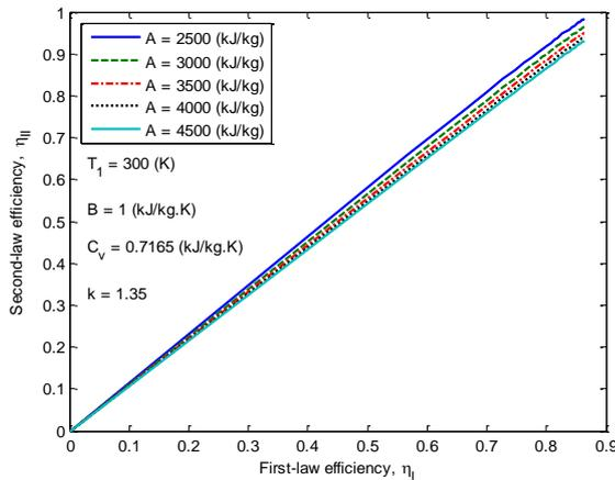
Fig. 3 Effect of  $A$  on the  $\eta_{II} - \eta_I$  characteristics
