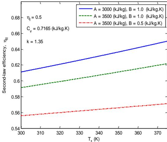
Fig. 2 Effect of  $A$  and  $B$  on the  $\eta_{II} - T_1$  characteristics
