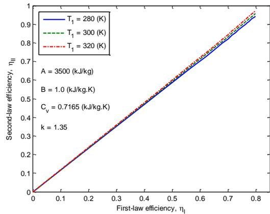
Fig. 5 Effect of  $T_1$  on the  $\eta_{II} - \eta_I$  characteristics
