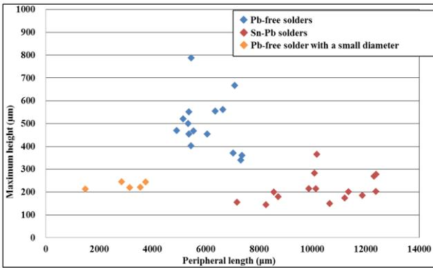
Fig. 5. Relationships between the maximum heights and the peripheral lengths of the respective melted solder samples.
