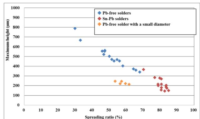
Fig. 3. Relationships between the maximum heights and the spreading ratios of the respective melted solder samples.
