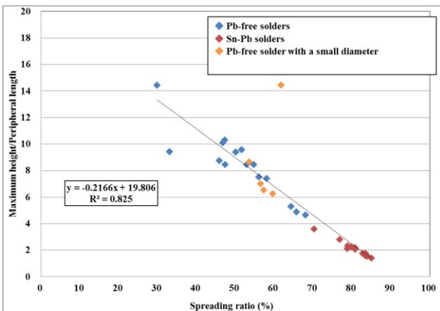
Fig. 7. Relationships between the ratios of the maximum heights to the peripheral lengths and the spreading ratios of the respective melted solder samples.
