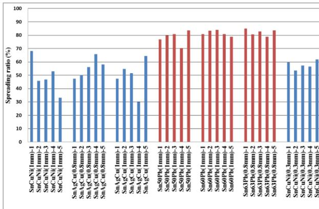
Fig. 1. Spreading ratio characteristics of the respective melted solder samples.
