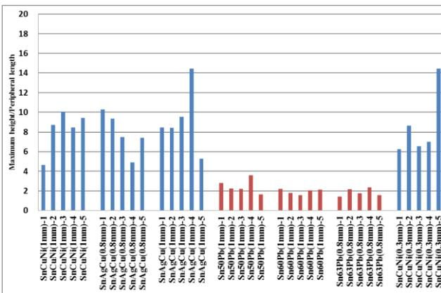
Fig. 6. Ratios of the maximum heights to the peripheral lengths of the respective melted solder samples.
