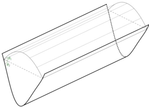
Fig. 4. Liquid in a channel with a constant cross-section. The two contact lines are assumed to be located on the horizontal plane. The contact angles  $\theta_1$  and  $\theta_2$  are above and below the horizontal plane, respectively.
