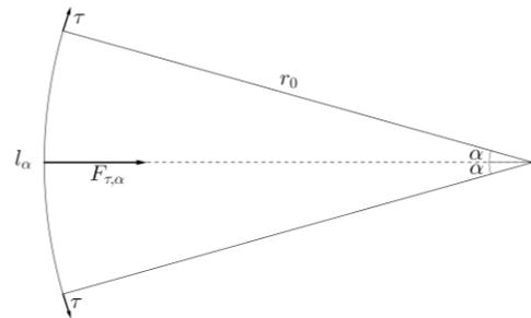
Fig. 1. A sector with central angle  $2\alpha$  and radius  $r_0$ . The arc is acted by the line tension  $\tau$  along the tangent direction and the arc length is  $l_\alpha$ .  $F_{\tau,\alpha}$  is the total centripetal force caused by the line tension  $\tau$ .
