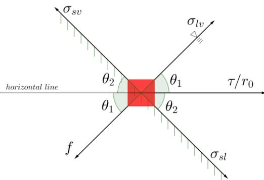
Fig. 3. The five forces caused by surface tension and line tension exert on an infinitesimal element around a triple contact line. In the horizontal direction, the summation of the five forces should be zero.
