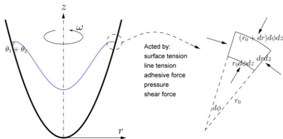
Fig. 5. Liquid rotates with an angular velocity  $\omega$ . For an infinitesimal element on the contact line, it is acted by the forces of surface tension, line tension, adhesive force, pressure, and friction in the horizontal direction.
