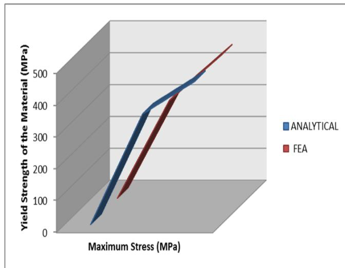
**Fig. 4.6** Comparison of analytical Method against FEA method for Stress on the Valve Gate
