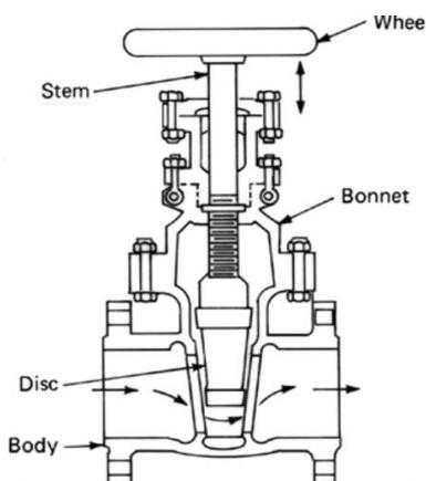
Fig. 1.1 schematic diagram of a gate valve
