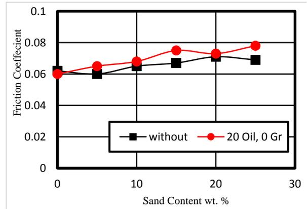
Figure 4 Effect of sand content on friction coefficient.
