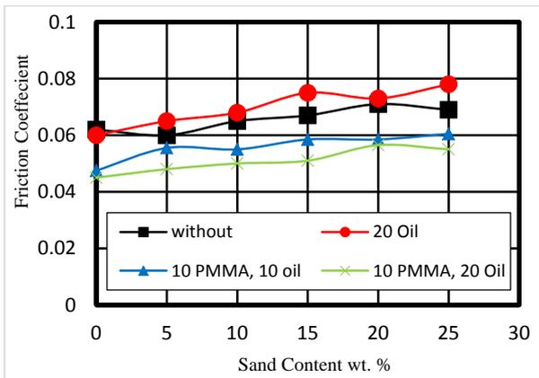
Figure 10 Effect of sand and PMMA contents on the coefficient of friction.
