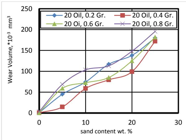
Figure 7 Effect of nano graphene content on wear volume of specimens.
