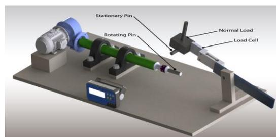
Figure 1 Layout of cross pin wear tester.
