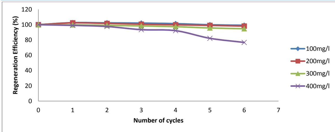
Figure 4. Effect of Microwave Regeneration cycles on the Regeneration efficiency of the spent activated carbons
