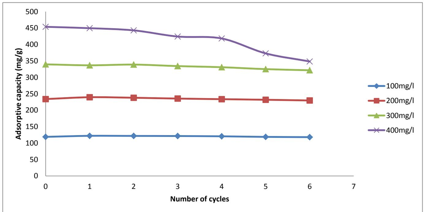
Figure 3. Effect of Microwave Regeneration cycles on the Adsorptive capacity of the spent activated carbons.
