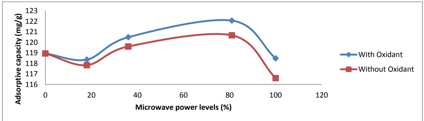
Figure 1. Effect of Microwave power level on the adsorptive capacity of regenerated carbon
