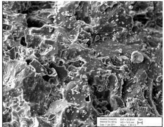
Fig. 11. The fracture surface image of iron-containing MgO material.
