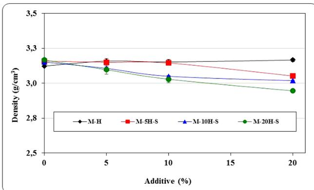
Fig. 2. Density values of MgO-hercynite-spinel Composite Refractories.
