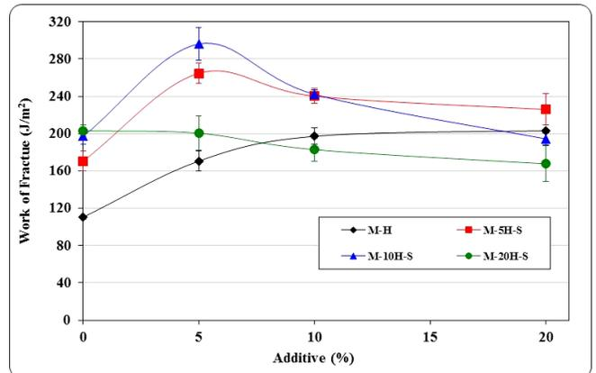
Fig. 7. Work of fracture values of MgO-hercynite-spinel Composite Refractories.
