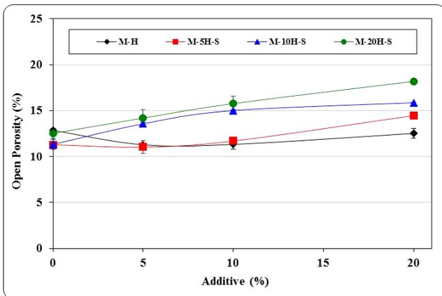
Fig. 1. Open porosity values of MgO-hercynite-spinel Composite Refractories.
