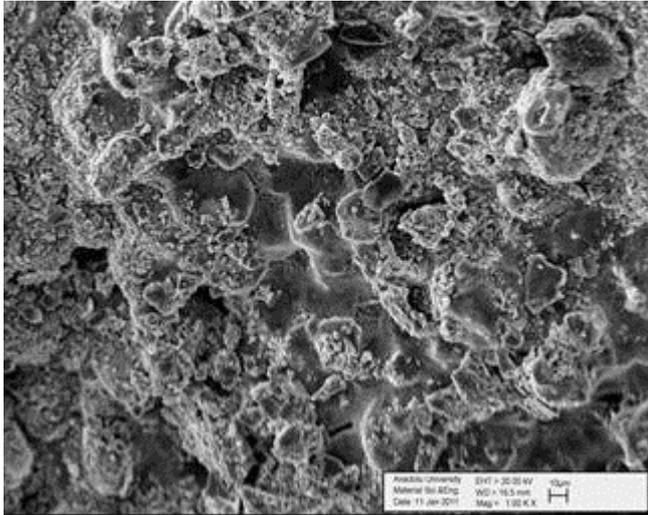
Fig. 13. The fracture surface image of M-10H%-5S% refractory material.
