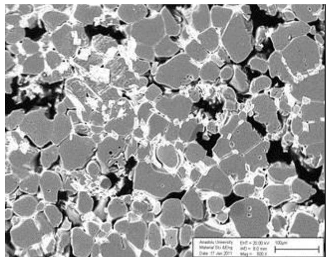
Fig. 8. The image of the microstructure of iron-containing MgO material (magnification: 500x).
