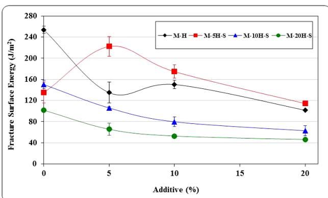
Fig. 6. Fracture surface energy values of MgO-hercynite-spinel Composite Refractories.
