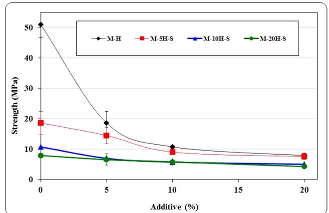
Fig. 3. Strength values of MgO-hercynite-spinel Composite Refractories.
