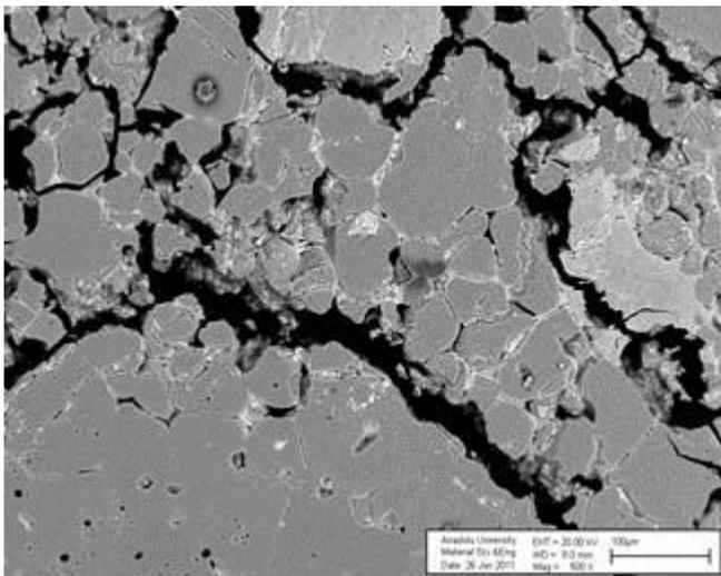
Fig. 10. The image of the microstructure of M-10H%-5S% material (magnification: 500x).
