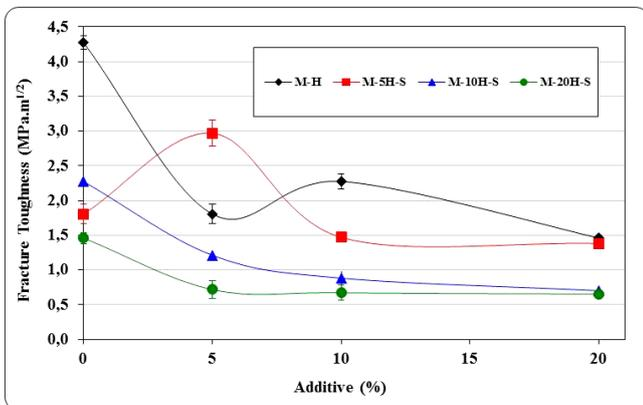
Fig. 5. Fracture Toughness values of MgO-hercynite-spinel Composite Refractories.
