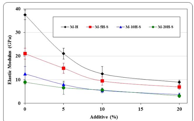
Fig. 4. Elastic Modulus values of MgO-hercynite-spinel Composite Refractories.
