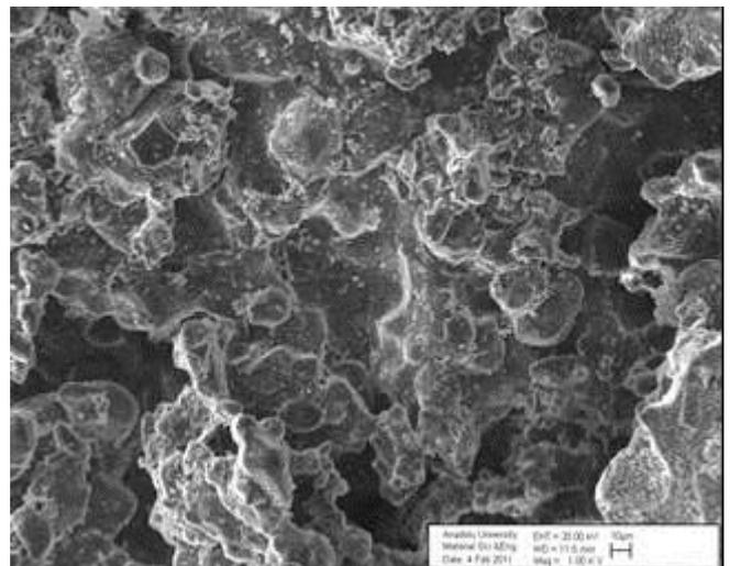
Fig. 12. The fracture surface image of M-10H% refractory material.
